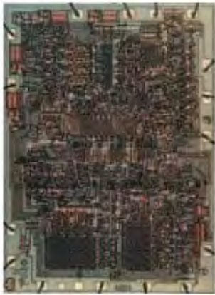
Intel® 4004 processor Initial clock speed: 108KHz Transistors: 2,300 Manufacturing technology: 10 micron
