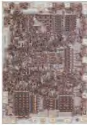
Intel® 8008 processor Initial clock speed: 800KHz Transistors: 3,500 Manufacturing technology: 10 micron
